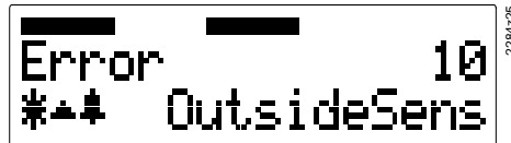
Example of own fault display
